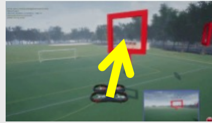
3D velocity command for drone to reach gate
