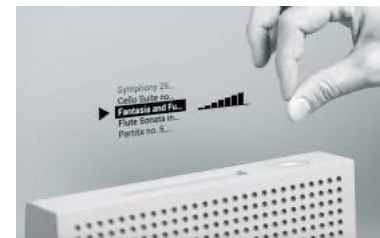
Soli: ubiquitous gesture sensing with millimeter wave radar (SIGGRAPH 2016)
