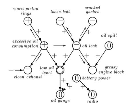
Qualitative influence of greasy engine block on worn piston rings: Greasy engine block is evidence for oil leak. Oil leak and excessive oil consumption can each cause low oil level. Oil leak explains low oil level and so is evidence against excessive oil consumption. Decreased likelihood of excessive oil consumption is evidence against worn piston rings. Therefore, greasy engine block is evidence against worn piston rings.
