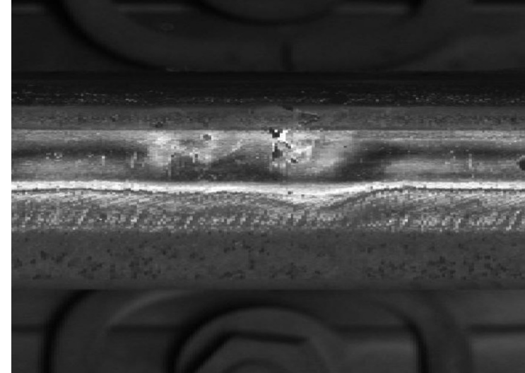
Surface defects & squats
